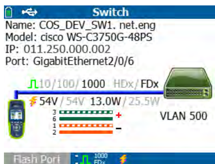
1 Gigabit link on copper with PoE on port 6
