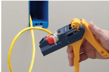
4. Ensure jack is completely and securely inserted in jack holder bed with IDC slots facing the blades.
