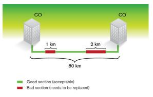
Contrary to the traditional approach, distributed PMD analysis breaks down the measurement results, effectively pinpointing the high-contributing sections of the link.
