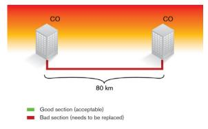
Traditional PMD measurement techniques provide a total link PMD value, but do not provide insight into which spans are causing the link to fail the test.
