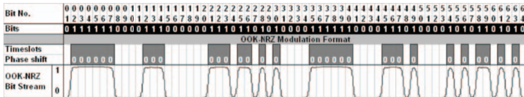
Diagram 16 – Example of NRZ format transmission
