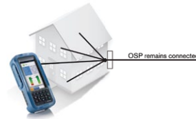
Figure 4. Using the Stressed Balance test to check the inside wiring
