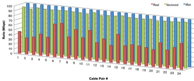
Figure 3. Actual versus vectored bit rates
