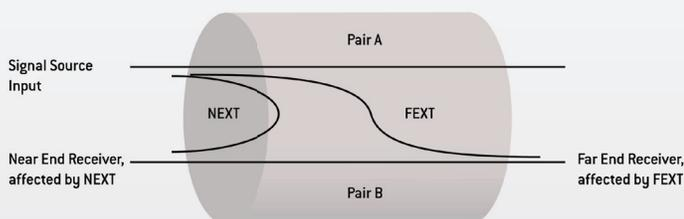
Figure 1. Crosstalk schematic
