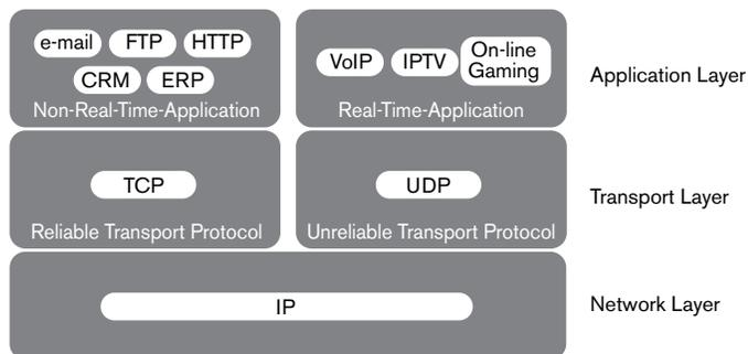
Figure 2. Applications running over TCP and IP protocols
