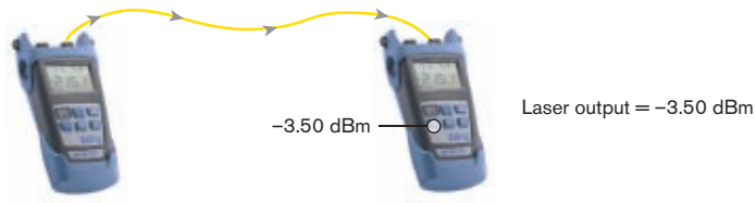
Figure 46 – dB (absolute): Measure the output power of a light source
