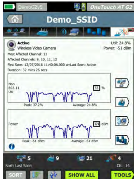
Figure 16. Detailed information about a specific interference source
