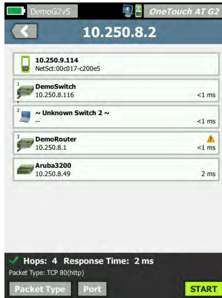
Figure 7. Path Analysis showing the path through switches from OneTouch AT to a client
