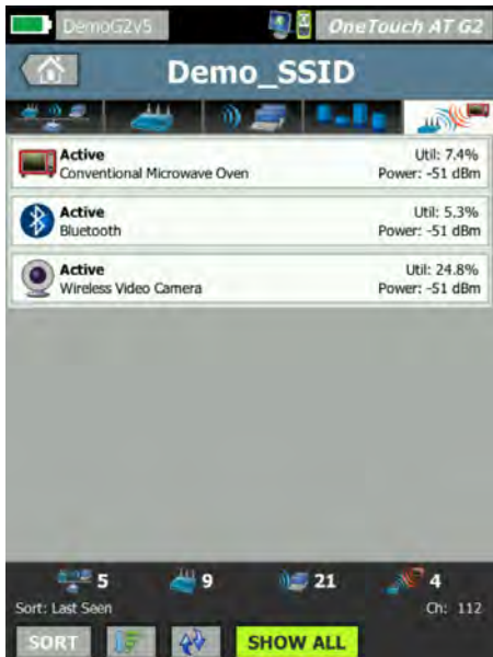
Figure 15. Unique Interferer analysis classifies sources of non-802.11
