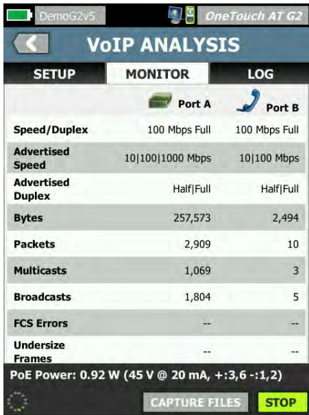
Figure 17. Inline VoIP analysis simplifies troubleshooting of desktop VoIP problems in real-time without TAPs or switch mirror ports
